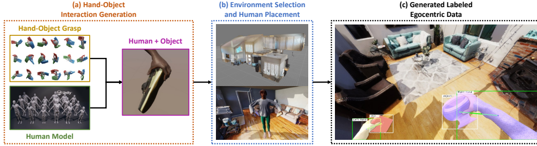
Figure 2. The proposed data generation pipeline. (a) An object-grasp pair is selected from DexGraspNet [9] and integrated with a randomly generated human model. (b) The human + object model is placed in an environment randomly selected from the Habitat-Matterport 3D dataset [6]. (c) Egocentric data of hand-object interactions is generated and automatically labeled.
